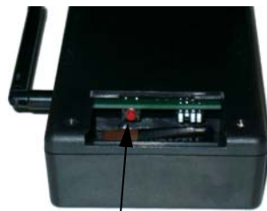
RED Push button for synchronizing both units
