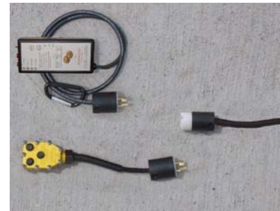
Connectors attached to Autopuller, original pull head and cord.
